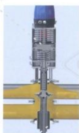
阀门开启 Valve Open
